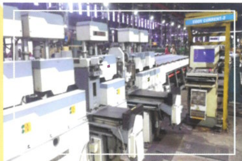
Eddy Current Testing for Bar
